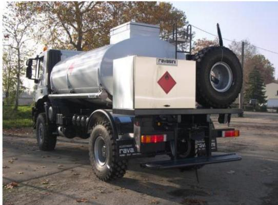
**Elliptical** section tank, one compartment, with capacity 11.000 l constructed entirely in steel sheet 4 mm thick both for the shells as for the dished heads and with dimensions suitable to the truck chassis supplied.
